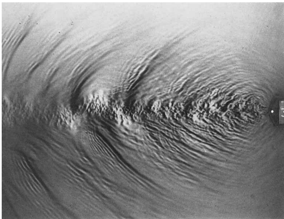
FIGURE 7. A shallow water-table simulation of the noise field, generated by the jet at 'supersonic' eddy convection speeds.
